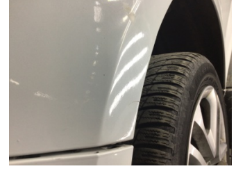
Çamurluk, sol, Çamurluk, sol > Çatlak
