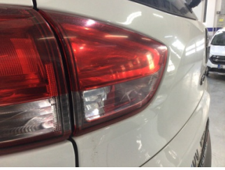
Arka lambalar, Arka lambalar, sol > Çatlak
