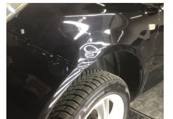
Çamurluk, sol, Çamurluk, sol > Ezik
