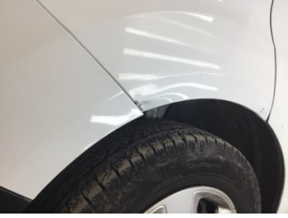
Çamurluk, sol, Çamurluk, sol > Ezik
