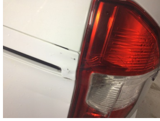
Arka lambalar, Arka lambalar, sol > Hasarlı
