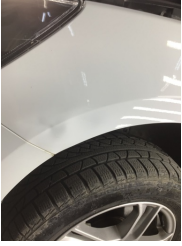
Çamurluk, sol, Çamurluk, sol > Ezik
