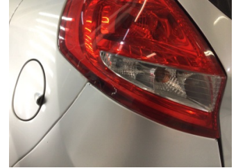
Arka lambalar, Arka lambalar, sol > Hasarlı
