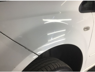
Çamurluk, sol, Çamurluk, sol > Ezik
