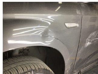
Çamurluk, sol, Çamurluk, sol > Ezik
