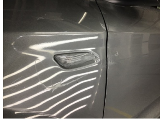
Çamurluk, sol, Çamurluk, sol > Ezik
