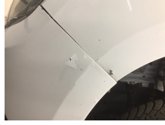
Çamurluk, sol, Çamurluk, sol > Ezik
