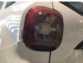
Arka lambalar, Arka lambalar, sol > Hasarlı
